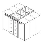
Blanking panels for different aisle containment heights to avoid air leakage at aisle.
