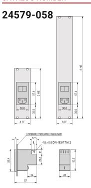
Front Panel for CompactPCI Systems with mounted Wide Range AC Input Module containing AC Plug, Fuse Holder and EMC Filter.
