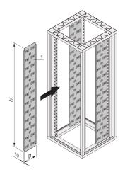
Eurorack Cable Panel allow cable management within the enclosure with cable ties and velcro. The unit is easily monted on the frame.
