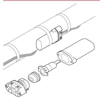
The nVent RAYCHEM E-150 is a cold applied low profile end seal. This universal end seal is designed to fit with all nVent RAYCHEM industrial self-regulating heating cables; BTV, QTVR and XTVR meaning simplified product selection and reduced inventory to stock. It can be used in applications with temperatures ranging from  $-55^{\circ}$ C to  $+200^{\circ}$ C. It is approved for use in hazardous areas.
