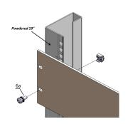
For standard grounding use a grounding nut and washer on at least one attachment point.
