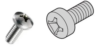
Pan head screws are a common head type of non-countersunk screw head used in self-tapping screws, self-drilling screws, and machine screws. They have wide heads, a flat bearing surface, high vertical, chamfered, or curved sides, and a flat or slightly domed top surface with a recessed socket.
