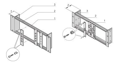
Module support is needed for assembly of partial width front panels with SUB-D-, ST type 3 or FDDI cut-outs, with or without strain relief rail.
