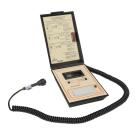
nVent RAYCHEM TraceTek TT-PTB-1000 is a battery powered portable device for testing individual lengths of sensing cable, up to 1000 m / 2000 ft. Useful for installation and maintenance of extensive systems.
