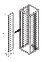
Vertical cable grid in different widths for Varistar free standing cabinets.
