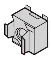
Cage nuts permit range of choice of nut and bolts sizes and easily replaced unlike pre-threaded holes. Cage nuts are easy to use on materials too thin or soft to be threaded.
