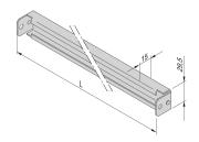
C-Rails are for better cable management. Installation generally behind the 19" uprights. They are compatible with standard cable clabs.
