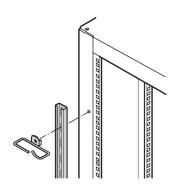
For assembly to the vertical uprights on the right and left hand side of the 19" plane; especially suited for cable eyes.
