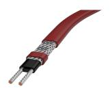
nVent RAYCHEM HTV self-regulating heating cable is designed for freeze protection or process temperature maintenance of pipes and vessels up to 205°C continuously, with a maximum exposure temperature of 260°C. The HTV cable has a solid construction with a high power retention (HPR) heating core and pressure extruded electrical insulation. It is then integrated with a robust metallic braid and a chemically resistant fluoropolymer outer jacket.
