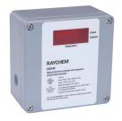
nVent RAYCHEM ECW-GF is an electronic line sensing or ambient thermostat with integrated 30 mA ground-fault protection, for self-regulating heating cables in pipe freeze protection, flow maintenance, frost heave protection or floor heating applications. Optional remote display panel, RAYCHEM ECW-GF-DP.
