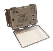
nVent RAYCHEM APS are a range of energy efficient control units for snow melting and gutter de-icing applications. Operating at various voltages, they can be used to control single heat tracing circuits or switch multiple circuits through a contactor.
