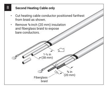
MARNING: Using the wrong splice can cause overheating. Use only the splice specified for the cable type.
