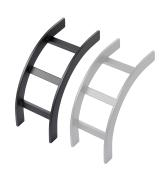
The Ladder Rack Curved Sections provide a vertical change in direction. They are made of 1-1/2 inch  $\times$  3/8 inch (38 mm  $\times$  8 mm) tubular steel with a painted or plated finish. Cross members are welded on the inside (inside bends) or outside (outside bends) of the section. They connect to straight section with butt-splice kits. They are also designed for category 5e, 6, 6A and fiber optic cable.
