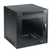
SOHO Cabinets are designed to house servers, networking equipment and phone and voice mail equipment under a desktop. Casters allow the cabinet to be easily moved for access. Equipment is passively cooled by air taken in from the front of the cabinet and expelled through fan cutouts in the rear, which can accept optional fans for warmer applications.
