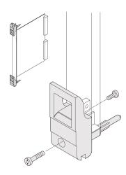
The inserter/extractor handle, type IET in accordance with IEEE 1101.10. 0,1" offset. Two of these handles can overcome a single lever force of 700 N (per pair).
