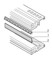
The contact strip makes contact bewteen horizontal rails. If two horizontal rails are mounted one above the other, the seals plus a metal strip enable EMC shielding.
