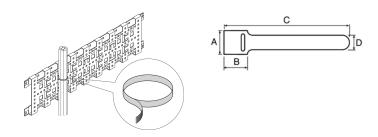
Velcro® Strip is one of the simplest cable bundling solutions. nVent SCHROFF Velcro® strip allows up to 90 mm diameter of wires.
