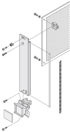
The stainless steel EMC gaskets are inserted into the lateral slots of the shieldable front panels (2 pieces per front panel).
