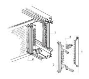
The coding is mounted on the side of a connector. With the Coding only the coded board can fit into the right slot.
