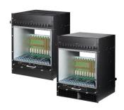
The nVent SCHROFF ATCA 450/40 FC Series is a family of AdvancedTCA Shelves that provide cooling and power per slot for 450 W blades. The backplane is verified in accordance to 40GBASE-KR4 for 40 Gbit Ethernet. Shelves with air flow from bottom to top as well as shelves with air flow from front to rear are available.
