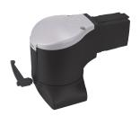
Syspend 180-Max Flange Elbow Coupling attaches directly to the enclosure for applications where a vertical tube is not required. It enables the enclosure to rotate 300 degrees and can be locked into a given position. The flange elbow coupling has a safety stop and maintenance-free bearings.
