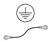
Enables IEC-compliant grounding, designed for Varistar CP.
