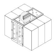
Profile that allows the easy fixing of aisle top covers. Increases aisle height and fixing point for accessories. Covers up to 4 racks.
