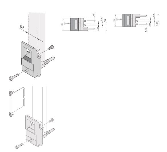
The inserter/extractor handle, type IET in accordance with IEEE 1101.10. 0,1" offset. Two of these handles can overcome a single lever force of 700 N (per pair).
