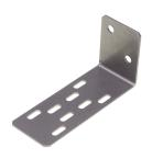
nVent RAYCHEM TraceTek TT-FFS-MOUNTING-BRACKET is an L shaped stainless steel bracket with cable ties, used to secure the fast fuel sensor nVent RAYCHEM TraceTek TT-FFS or the nVent RAYCHEM TraceTek TT-MINI-PROBE probe vertically on open flat areas.
