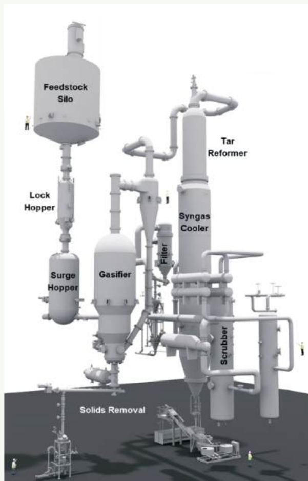
Figure 5 S1000: an integrated gasification system for syngas production from woody biomass
