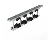
This busbar support, EUBS, is available for one, two, or three bars up to  $120 \times 10$  mm. The support can be mounted either at the top or bottom of the enclosure. It is available off the shelf and tested according to IEC 61439. This support is required when a high level of mounting flexibility is required.
