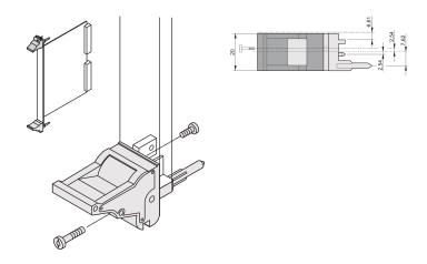
The inserter/extractor handle, type IEL in accordance with IEEE 1101.10. 0,1" offset Two of these handles can overcome a single lever force of 700N (per pair).
