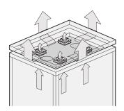
Top covers with fans are compact active cooling units which do not consume rack space. Eurorack fantray is delivered without the fans for raised top covers.
