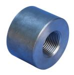
The nVent LENTON brand of cryogenic reinforcement splicing systems should be specified whenever cryogenic-grade reinforcing bar is used, or during normal operating or emergency conditions where the temperature falls below - 20 °C (-4 °F). By combining the nVent LENTON taper-threaded couplers with state-of-the-art materials, we have developed one of the slimmest couplers on the market, while still maintaining top performance. Typical construction projects include LNG and LPG storage tanks.
