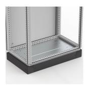
This steel bottom plate, CBP, comprises of three pieces, available off the shelf, and should be used when the bottom part of the enclosure must be covered. The enclosure's stated protection degree will remain intact. The plates can be removed easily to allow for mounting of cabling accessories.
