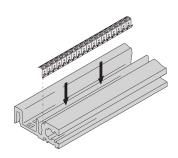
Stainless steel gasket is clipped into a groove of horizontal rail and enables contact to the cover plate.
