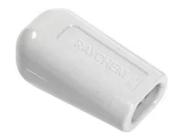
nVent RAYCHEM RayClic-E-XX end seals are a simple, fast and reliable end termination developed for select nVent RAYCHEM XL-Trace, IceStop and HWAT self-regulating heating cables. No heat guns or wire stripping are needed, because silicone gel technology is used to make the electrical termination.
