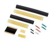
nVent RAYCHEM CCE series are cold lead connection and end seal kits for use with select nVent RAYCHEM self-regulating trace heating cables with modified polyolefin or Fluoropolymer outer jacket and cold lead cables with overall diameter between 6-11 mm. Each kit contains crimps, heat shrinkable sleeves and end seals. Requires wire stripping and a heat gun.
