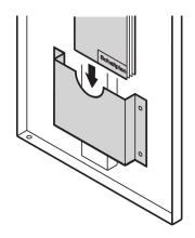
Document pockets for storage of documents and circuit diagrams, with easy mounting with double sided adhesive tapes.
