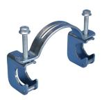
The Quick Grip Lateral Brace, part of the nVent CADDY line of fire sprinkler bracing systems from nVent, is designed to help simplify installations when bracing service pipe for seismic or other catastrophic events. It features an innovative design for quick attachment of brace pipe to service pipe saving time and money.
