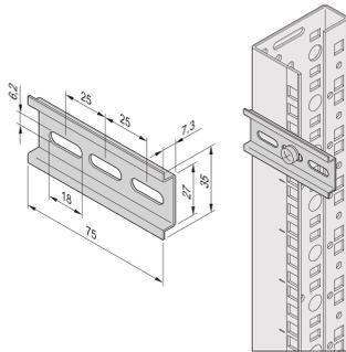
DIN rail for thermostat or hygrostat clamping.
