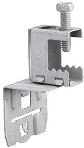
The Improved nVent CADDY Cat HP Mod Clip J-Hook with BC Swivel Beam Clamp offers both easy beam flange installation and 360-degree rotation for versatile cable routing. By eliminating the need for screws, rivets or special tools during assembly, installation time and cost is reduced. A simple clip onto nVent CADDY Cat HP components ensures a secure hold—ultimately enhancing rigidity and stability while minimizing inventory impact and providing flexibility on the job site.
