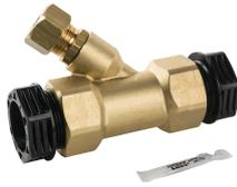
nVent RAYCHEM Y-Connection for in-pipe pipe freeze protection applications. Suitable to use with ETL and FrostGuard self-regulating heating cable. For 25 or 32 mm pipe diameter.
