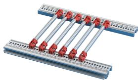
Plastic end pieces for individual multi-piece guide rails with plastic or extrusion mid-piece. Available as Standard, Accessory or 4.4" PCB types. End pieces can be optional equipped with a ESD clip, which ensures conductive contact between PCB and horizontal rail. Suitable for RatiopacPRO/-AIR, PropacPRO, CompacPRO and EuropacPRO.
