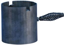
The crucible extension is a cylindrical steel tube that extends the graphite crucible, allows for gas expansion and retains the molten filler material. The crucible extension helps ensure containment of the exothermic reaction.
