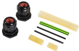
nVent RAYCHEM EM2-XR CE32-02 is a connection and end seal kit for use when circuits are greater than 32 A and the cold lead cable is limited to 5 m. In this case, an intermediate connection is made to a junction box.
