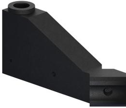
Angular extended side fill horizontal pouring basins are used when interferences of the structure will not allow top filling of the sleeve and the interferences are directly next to the tap hole in the sleeve.
