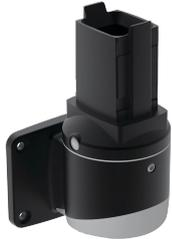
Syspend 281-Max Vertical Wall Joint mounts the suspension system to a vertical surface, allowing the tube to extend vertically. The arm can be rotated 300 degrees. Includes a safety stop and maintenance-free bearings.
