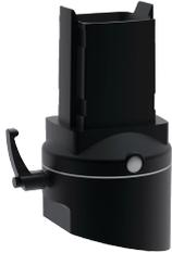
Use Angled Coupling Tilted Backward to mount enclosure at a 15-degree backward angle. Enclosure can be rotated 300 degrees and locked in position. Includes safety stop and maintenance-free bearing.
