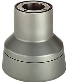
CS480 Swivel Base Bracket Coupling Internal mounts the enclosure directly to horizontal surfaces, enabling 340-degree enclosure rotation. Base mounting hardware is hidden. Maintenance-free bearings.
